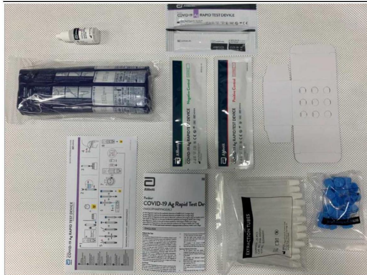
Figure 3: Overview of Panbio™ COVID-19 Ag Rapid Test Device kit components (Ref. 41FK10). Note: in this example, only one packaged test device is shown, while a kit would contain 25.
